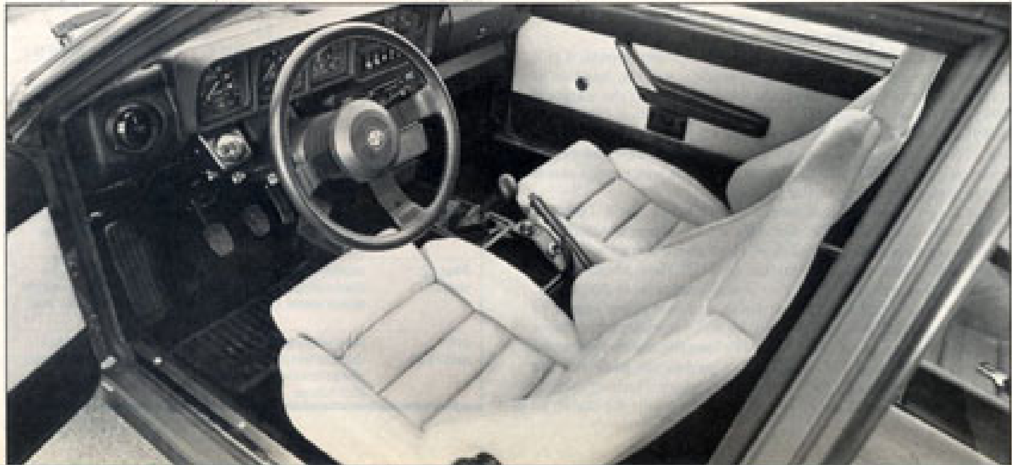
Callaway Twin Turbo has the optional leather interior and boost gauge added below speedometer.
